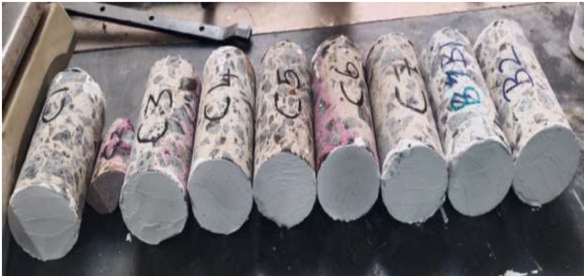
Figure.1 Concrete core samples
