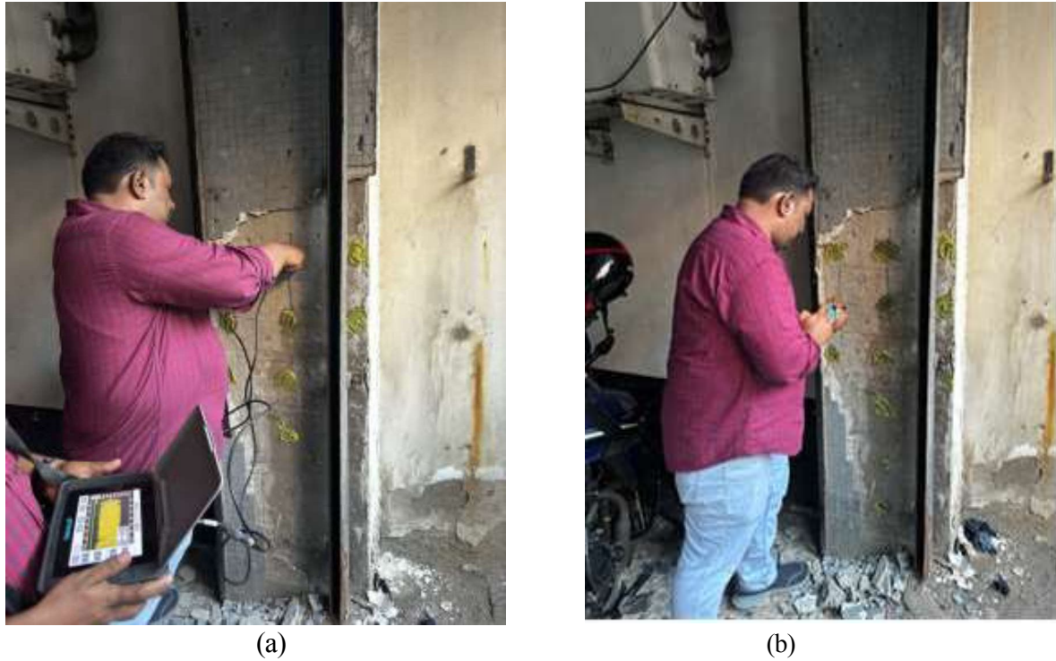
Figure.7 (a) UPV test and (b) Rebound hammer test at location C7
