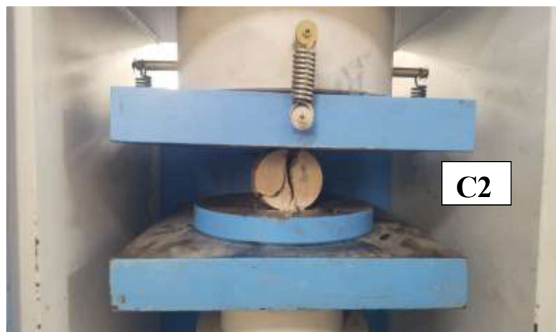
Figure.18 Split tensile testing of core cut sample for carbonation test
