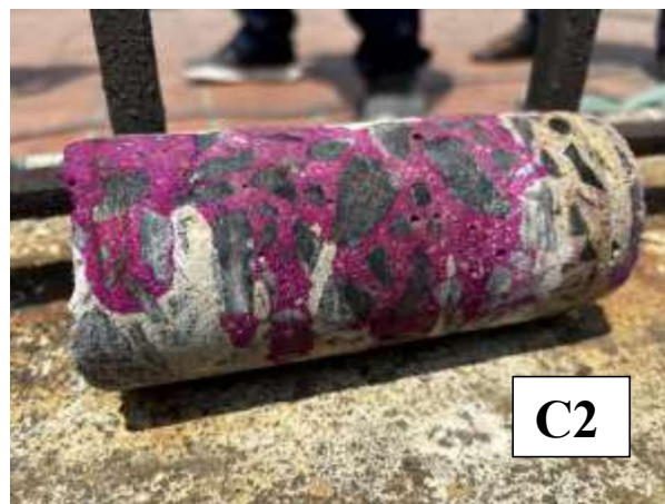
Figure 16. Carbonation test conducted at site for C2 sample
