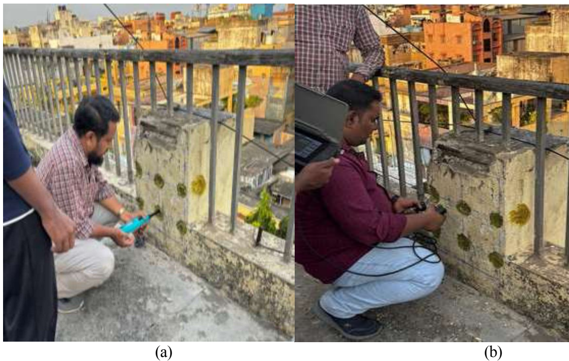
Figure.8 (a) Rebound hammer test and (b) UPV test at location C3
