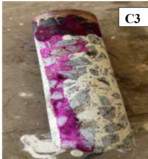
Figure 17. Carbonation test conducted at site for C3 sample
