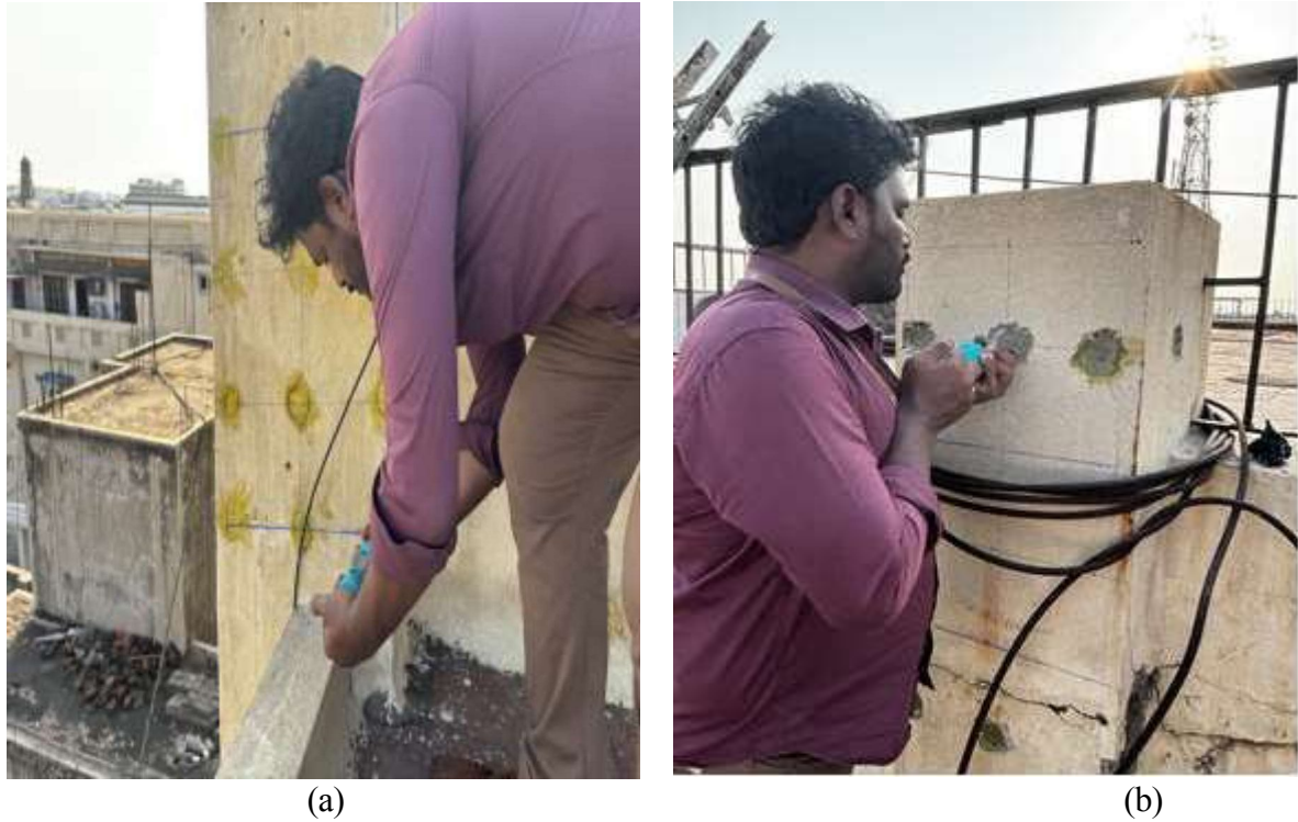
Figure.11 Rebound hammer test at location C1 & C1'
