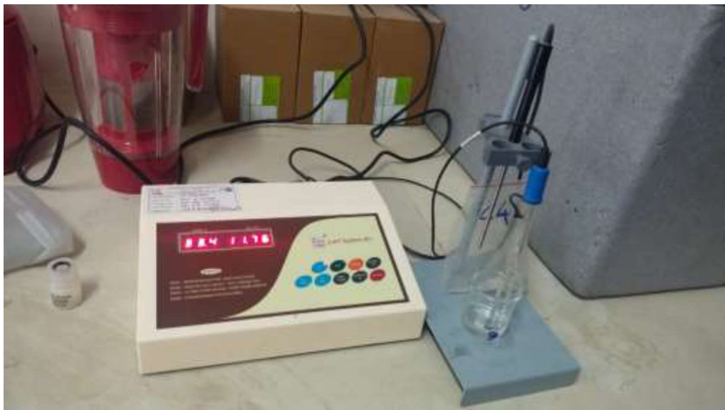
Figure.13 pH experimental setup at lab
