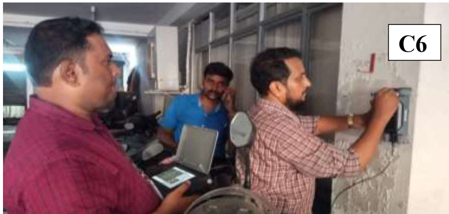
Figure.5 Locating rebar at C6 location using profoscope
